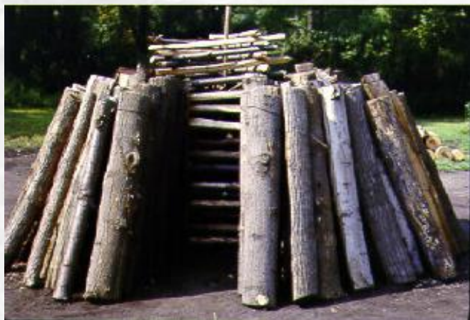
Stack with central chimney
