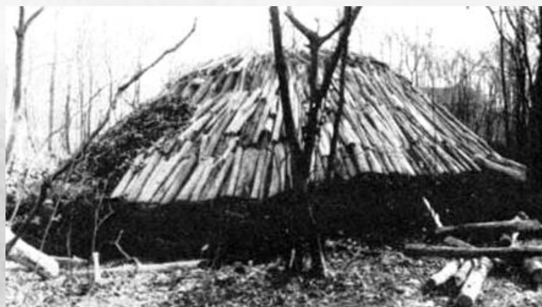
Stack being covered with dirt to cut off air
