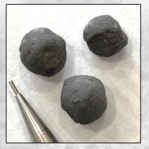
Hematite Pellets for Blast Furnace Feed
